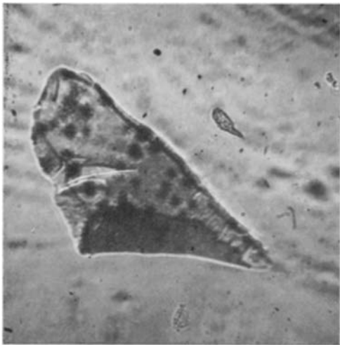
Figure 2 Star-shaped inclusions of \text{CaF}_2 crystals in glass (without crossed nicols) ( \times 160 ).
