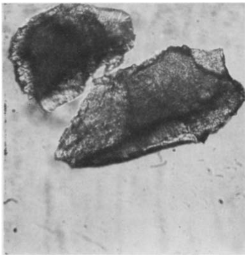
Figure 3 Appearance of glass compositions with more than 35% \text{CaF}_2 after quenching (without crossed nicols) ( \times 160 ).
